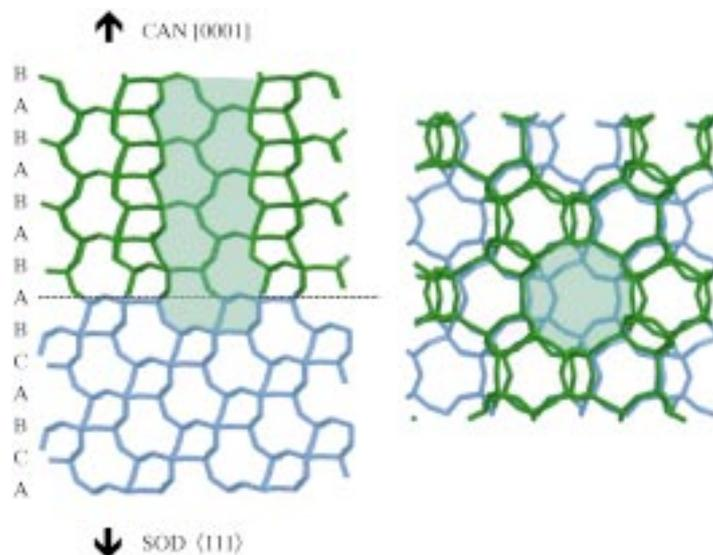
Figure 1. A model of heteroepitaxial growth of cancrinite on sodalite. The stacking sequence along the cancrinite [0001] direction is ABABAB (top), and that along the sodalite  $\langle 111 \rangle$  direction is ABCABC (bottom). A composite view down the cancrinite [0001]/sodalite  $\langle 111 \rangle$  direction is shown on the right. The shaded areas represent the connection of a sodalite cage and a 12-membered ring cancrinite channel on the left, and a single sodalite cage on the right.
