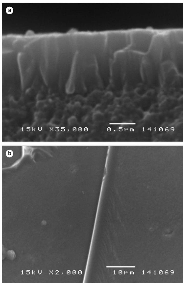
Fig. 1. SEM images of (a) cross-section of Type B MFI membrane, (b) top view of Type B MFI membrane showing a crack sealed with silica.
