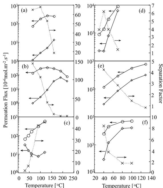
Fig. 4. Separation factors and permeation fluxes through faujasite membrane at different temperatures, for (a) 5 kPa benzene/5 kPa cyclohexane, (b) 5 kPa benzene/5 kPa *n*-hexane, (c) 5 kPa toluene/5 kPa *n*-heptane, (d) 50.5 kPa propylene/50.5 kPa propane, (e) 50.5 kPa ethylene/50.5 kPa ethane, and (f) 50.5 kPa ethylene/50.5 kPa methane binary mixtures. (○) flux of the higher-permeating hydrocarbon; (◇) flux of the lower-permeating hydrocarbon; (×) selectivity factor.
