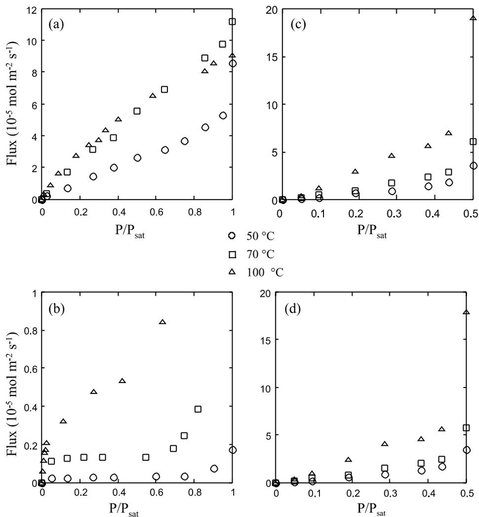
Fig. 2. Permeation fluxes through Type A MFI membrane at different temperatures: (a) single-component *p*-xylene, (b) single-component *o*-xylene, (c) binary *p*-xylene, and (d) binary *o*-xylene.
