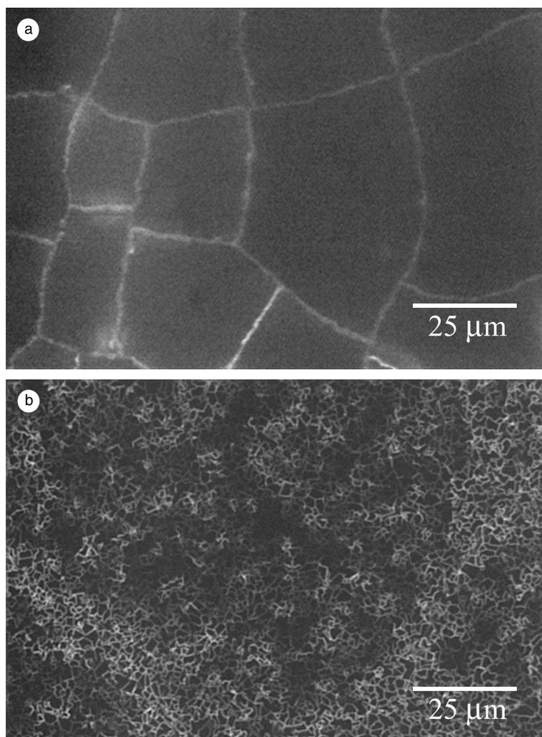
Fig. 3. Confocal microscope images of MFI membranes infiltrated with fluorescein dye: (a) Type B membrane showing cracks but no grain boundaries, and (b) Type A membranes showing grain boundaries between zeolite crystals.
