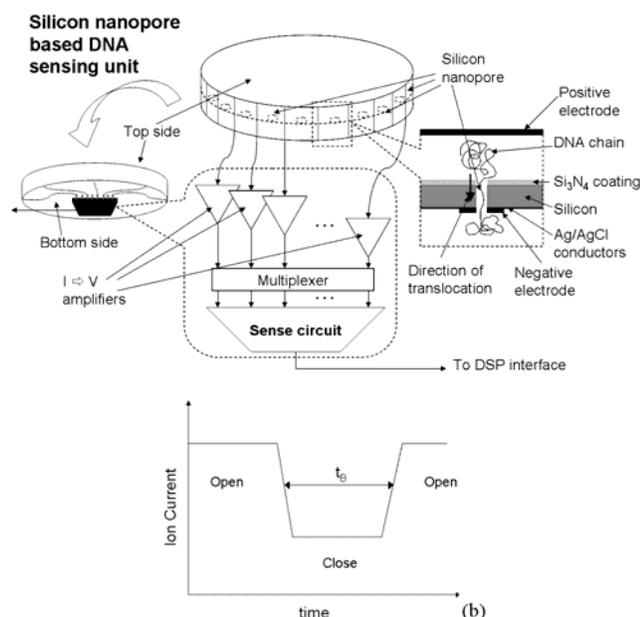
**Figure 1. Internal diagram and the operating principle of the sensor: In ‘open’ mode, the pore permits a high current. During translocation, the current is reduced to a low level due to partial pore blockage by the molecule. The blockage duration ( $t_B$ ) correlates to the molecule length.**
