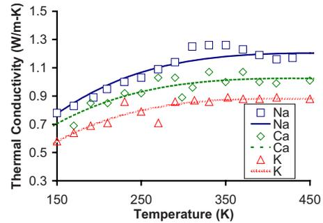
FIG. 4. (Color online) Measured (symbols) and model-fitted (curves) thermal conductivity of LTA zeolite films containing different nonframework metal cations ( $\text{Na}^+$ ,  $\text{Ca}^{2+}$ , and  $\text{K}^+$ ).
