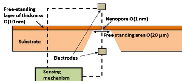
Fig. 1 Solid state END geometry and design considerations.
