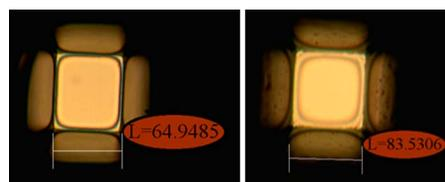
**Fig. 13** Optical images of two devices (50-nm silicon nitride) after backside wet etch. The window dimensions shown are in micrometer.
