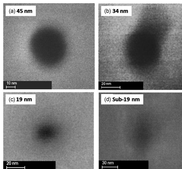
**Fig. 12** SEM images of a single nanopore undergoing ALD cycles, as shown in Fig. 11 (pore 2). The nanopore size is reduced in a controlled manner and with nanometer scale precision.
