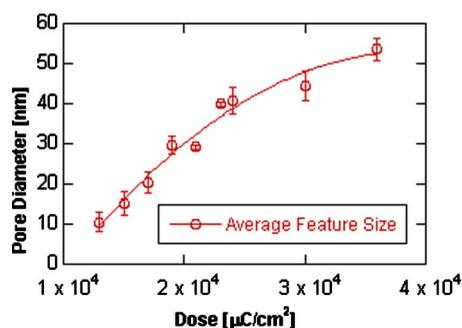
**Fig. 3** Average pore size as a function of dose in 100-nm ZEP 2:1 after development. The curves are only a guide to the eye.
