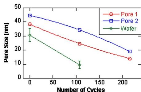
**Fig. 11** Nanopore size as a function of number of ALD cycles for two pores (with a deposition rate of  $0.58\text{-}\text{\AA}$   $\text{Al}_2\text{O}_3$  per cycle) and an entire wafer (with a deposition rate of  $0.9\text{-}\text{\AA}$   $\text{Al}_2\text{O}_3$  per cycle). The curves are only a guide to the eye.
