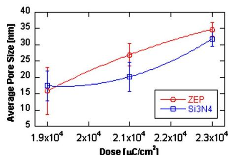
**Fig. 7** Pore size as a function of dose before and after pattern transfer for single-shot dosing. The curves are only a guide to the eye.
