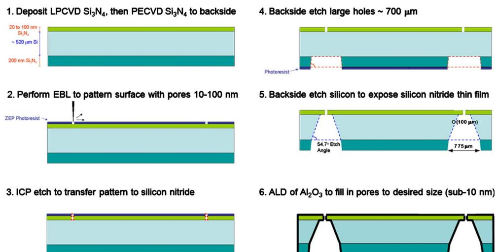
Fig. 2 Major process steps in tunable fabrication of arrays of nanopores on a wafer.
