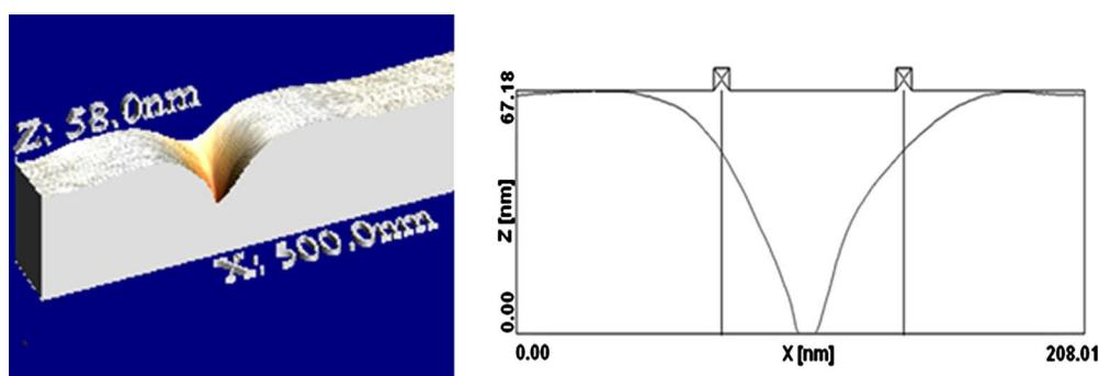
**Fig. 10** AFM depth profile (left) and the profile cross section (right) of a 50-nm to 60-nm pore in 16-nm thin silicon nitride film.
