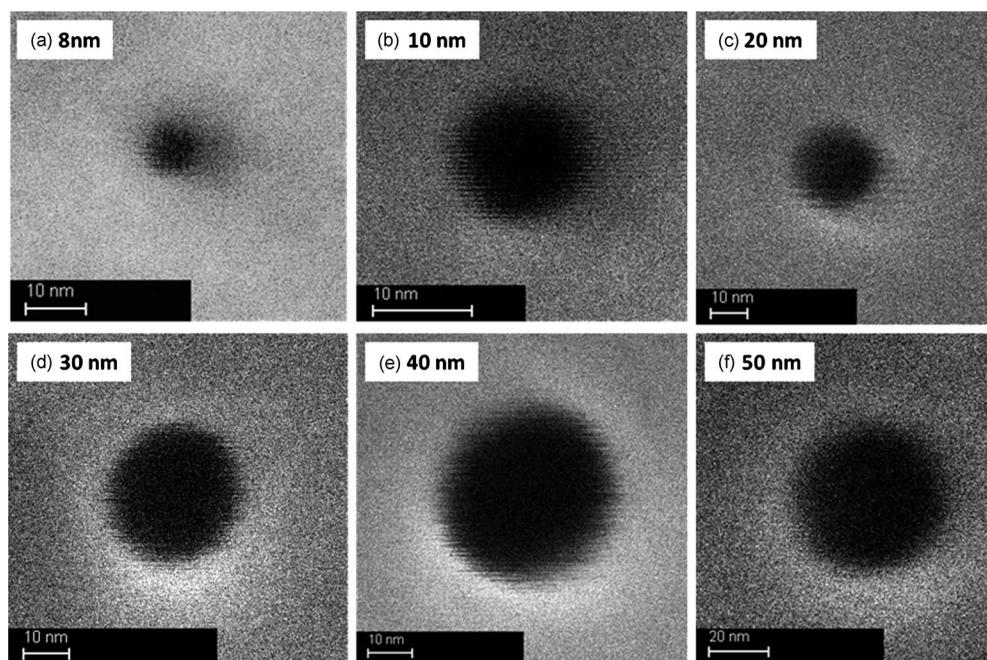
**Fig. 4** High-resolution SEM images of nanopores of varying sizes patterned in 100-nm-thick ZEP2:1 resist films at different doses. From (a) to (f), pore sizes of 8, 10, 20, 30, 40, and 50 nm (see Fig. 3 for corresponding electron doses).
