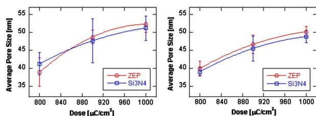
**Fig. 6** Pore size as a function of dose for two wafers after identical processing. The curves are only a guide to the eye.
