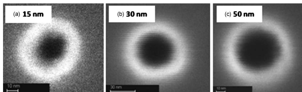
**Fig. 8** Nanopores of various diameters transferred from the e-beam resist to the silicon nitride films; (a) and (b) in 16-nm silicon nitride and (c) in 7-nm silicon nitride.
