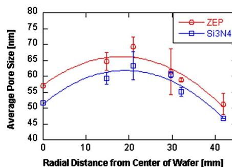
**Fig. 5** Patterned nanopore size as a function of radial distance on the wafer before and after pattern transfer. The curves are only a guide to the eye.
