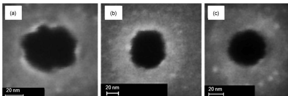
**Fig. 9** Three isolated pores unmarked by calibration features showing the types of imperfections that can occur during processing: (a) and (b) jagged pores created by unoptimized doses in 7-nm and 16-nm silicon nitride, and (c) good-quality circular pore created by optimized dose in 7-nm silicon nitride.
