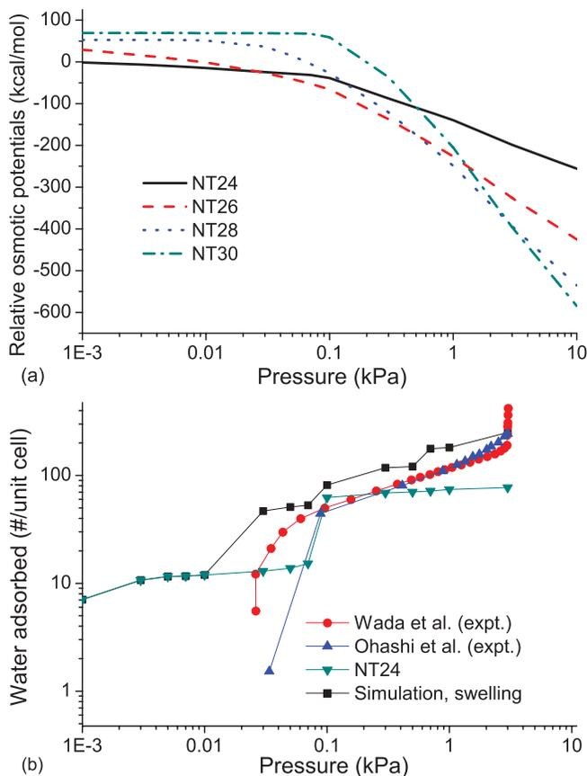
FIG. 4. (a) Relative osmotic potentials of NT24, NT26, NT28, and NT30 and (b) new adsorption isotherm obtained from thermodynamics analysis compared with experiments (Refs. 27 and 28) and that of NT24.
