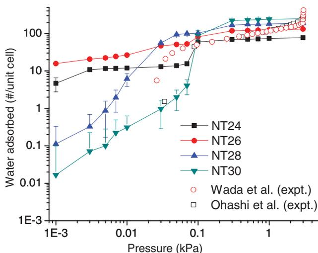
FIG. 2. Calculated adsorption isotherms of water in hexagonally packed aluminosilicate NTs, compared with experimental results from Wada and Yoshinaga (Ref. 27) and Ohashi *et al.* (Ref. 28).
