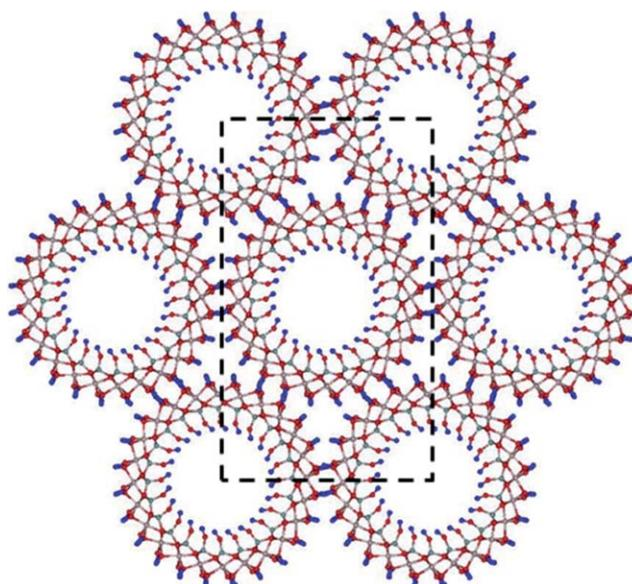
FIG. 1. Structure of hexagonally packed aluminosilicate NTs viewed along the axial direction with 24 Å spacing. Dotted lines indicate the simulation volume. Blue: hydrogen, red: oxygen, pink: aluminum, grey: silicon.
