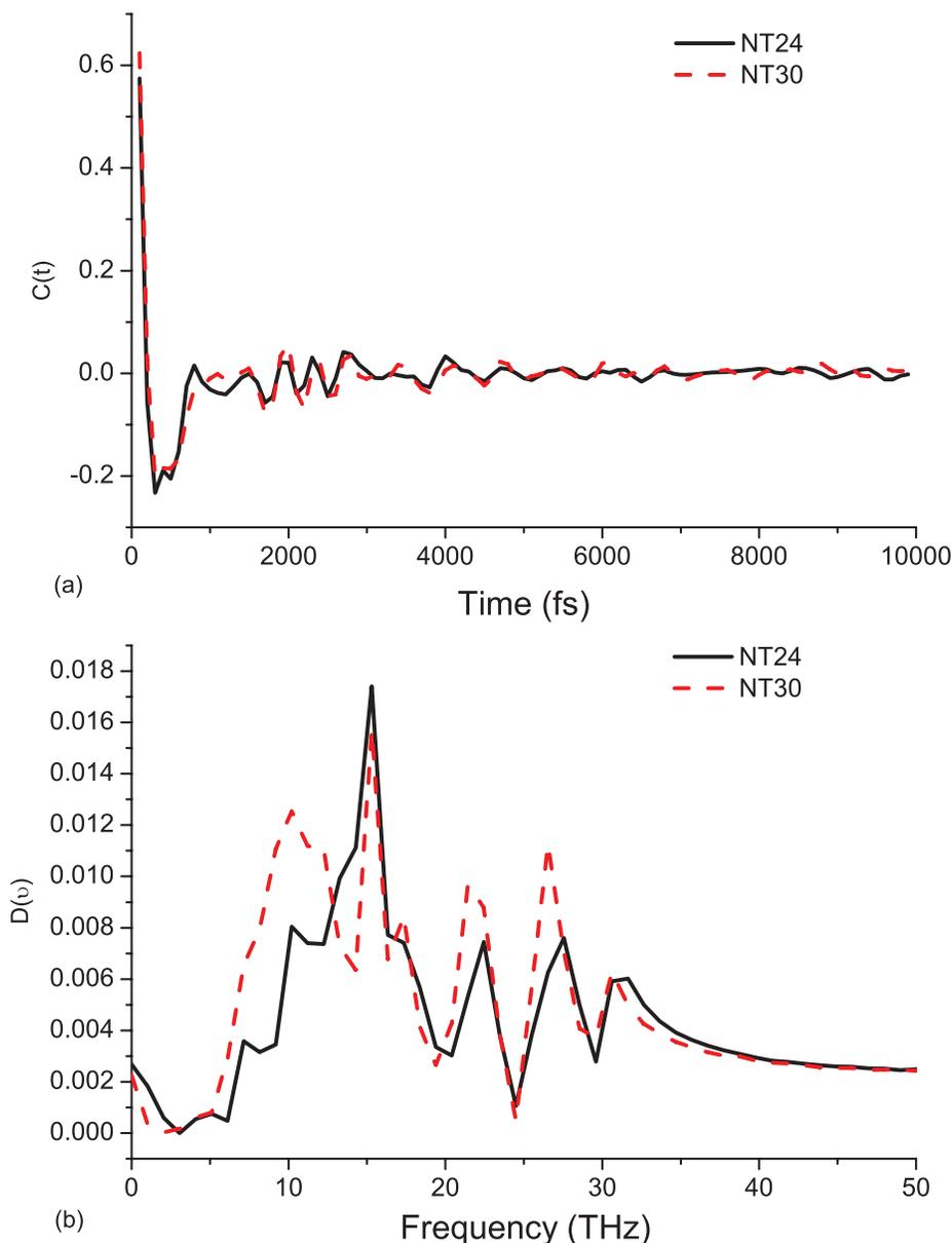
FIG. 3. (a) Velocity autocorrelation function and (b) vibrational density of states for NT24 and NT30.
