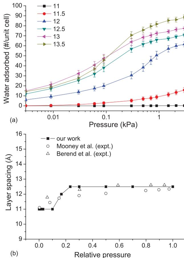
FIG. 5. (a) Water adsorption isotherms and (b) swelling curves from experiments (Refs. 30 and 32) and our prediction.
