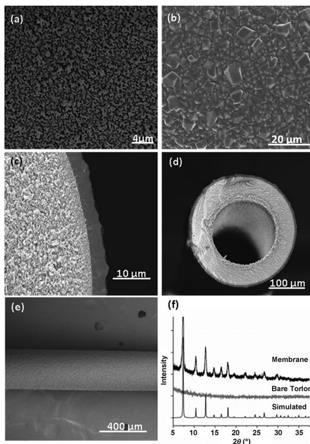
**Figure 2.** SEM images of: a) the ZIF-90 seed-layer, b) top view and c,d) cross section views of the polycrystalline ZIF-90 membrane after secondary growth, e) low-magnification view showing complete coverage of the fiber surface by the ZIF-90 membrane, and f) XRD patterns of bare Torlon and the membrane.
