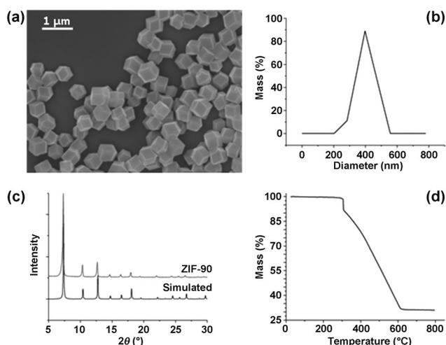
**Figure 1.** a) SEM Image of ZIF-90 nanocrystals, b) particle size distribution estimated from dynamic light scattering (DLS) analysis, c) XRD patterns of ZIF-90 particles and comparison to the simulated pattern of the ZIF-90 structure, and d) thermogravimetric profile of ZIF-90 particles.
