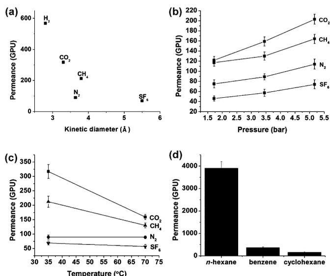
**Figure 3.** Permeances of gases at a) 35 °C and 50 psia as a function of kinetic diameter, b) 70 °C as a function of pressure, c) 50 psia as a function of temperature, and d) permeances of hydrocarbons at 22 °C by pervaporation. Error estimates were obtained as standard deviations from independent permeation measurements on 3 or more samples, and varied from 6% for N<sub>2</sub> to 11% for cyclohexane.
