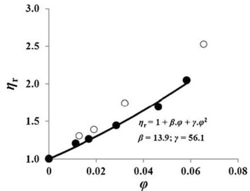
**Fig. 8** A quadratic fit to the relative viscosity versus volume fraction of uncalcined ST MFI particle suspension to determine the intrinsic viscosity,  $\beta$ , and the interaction term coefficient,  $\gamma$ , for MFI particles. *filled circle*, uncalcined MFI; *unfilled circle*, calcined MFI
