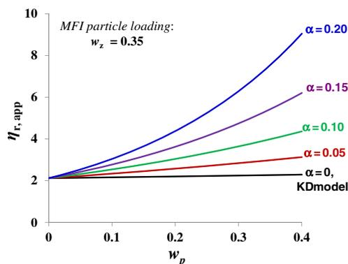
**Fig. 5** The apparent relative viscosity of suspensions with 35 wt% MFI particles in suspending Ultem/NMP media with varying nominal weight fractions of polymer for different values of the absorption parameter  $\alpha$
