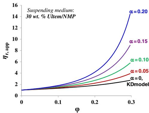
**Fig. 4** The apparent relative viscosity of suspensions of MFI particles in a 30 wt% Ultem/NMP solution for different values of the absorption parameter  $\alpha$
