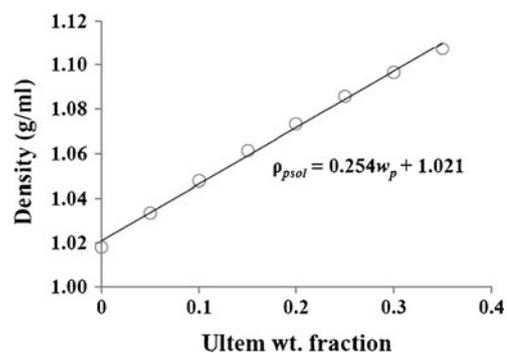
**Fig. 2** Density of Ultem/NMP solutions at  $50 \text{ }^\circ\text{C}$  as a function of polymer concentration
