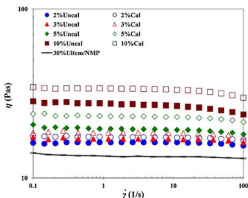
**Fig. 7** Flow curves for polymer solution and suspensions of uncalcined and calcined MFI particles. *Unfilled* and *filled* symbols represent porous and nonporous MFI particles, respectively, while the different *geometric symbols* indicate MFI concentration: *circle* (2 wt% MFI), *triangle* (3 wt% MFI), *diamond* (5 wt% MFI), *square* (10 wt% MFI)
