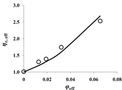
**Fig. 9** Effective relative viscosity versus effective volume fraction for calcined MFI particle suspensions (volume fraction corrected with  $\alpha = 0.18$ ); line represents model predictions using  $\alpha = 0.18$ . Effective relative viscosity only accounts for the effect of solvent absorption to suspension viscosity
