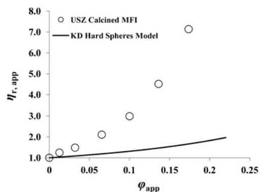
**Fig. 6** Relative viscosity as a function of particle volume fraction; large deviation between calcined MFI suspension and the Krieger–Dougherty hard sphere model prediction is observed
