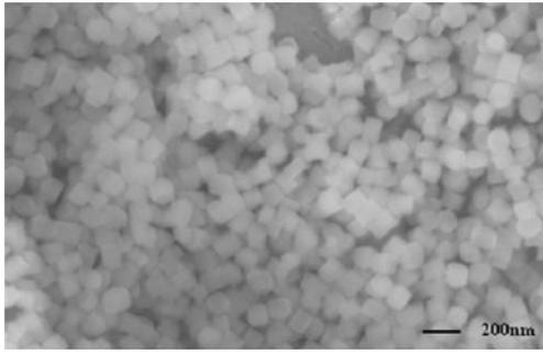
**Fig. 1** SEM micrograph of pure silica MFI zeolite particles
