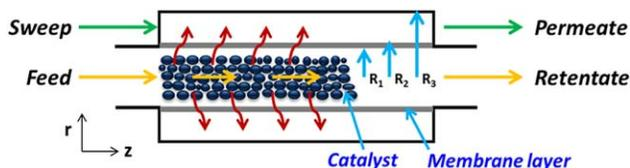
**Figure 1. Schematic of a PDH PBMR.**
