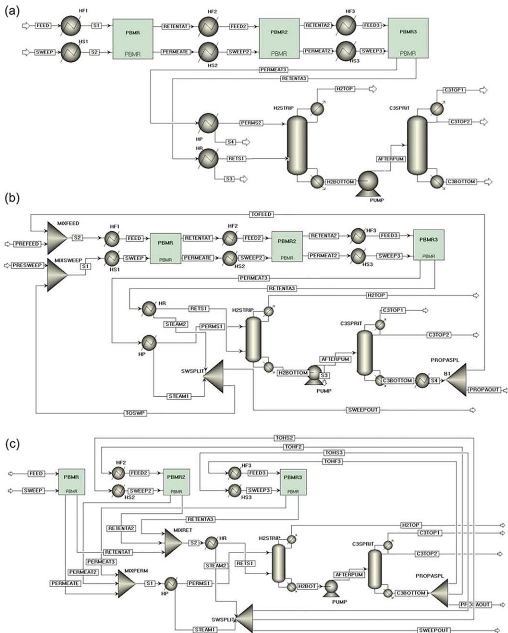
**Figure 2. ASPEN flowsheets of PDH plant using 2-D nonisothermal PBMR model with downstream separation: (a) single-pass, (b) simple recycle, (c) recycle with reactor stages in parallel and recycled propane distributed equally to the second and third stages.**
