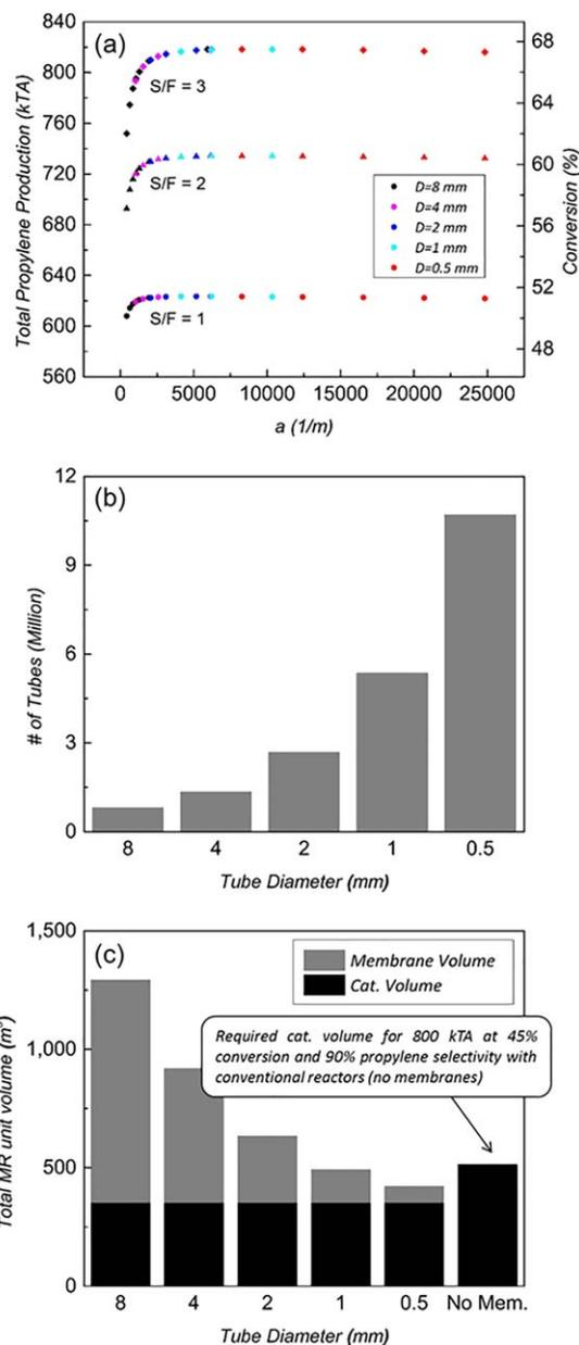
**Figure 5.** (a) Propylene production rate and conversion as a function of membrane surface area per unit volume,  $a$ . (b) Comparison of required number of membrane tubes for different target conversions (or propylene production rates) with a fixed  $4000 \text{ kmol h}^{-1}$  propane feed. (c) Comparison of required membrane reactor volume for 800 kTA propylene production ( $S/F = 3$ ).
