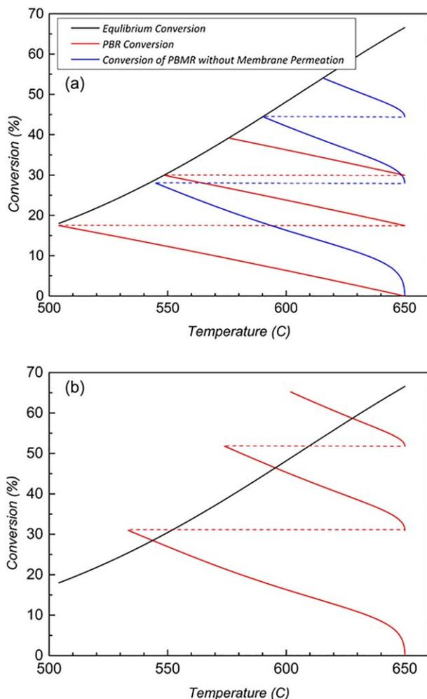
**Figure 7. (a) Adiabatic operating line of PBR and zero-permeance PBMR configuration (S/F = 3). (b) Adiabatic operating line of PBMR (S/F = 3) along the three reactors. The dashed lines depict the reheating of retentate streams in interstage heaters.**
