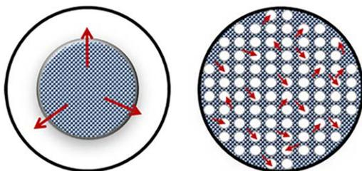
**Figure 4.** Schematic of PBMR configuration using a tubular membrane with packed catalyst in the bore side (left), and a hollow fiber membrane bundle with catalyst on the shell side (right). The shaded areas and arrows represent packed catalyst and the direction of gas permeation (from the catalyst toward the tube/fiber surface), respectively.
