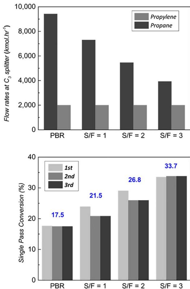
**Figure 10.** (a) Flow rates entering  $C_3$  splitter and (b) single-pass conversions for the reactors-in-parallel system shown in Figure 2c.
