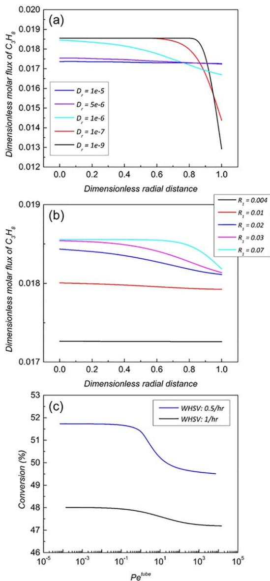
**Figure 3.** (a) Effect of dispersion coefficient ( $D_t$ ,  $\text{m}^2 \text{s}^{-1}$ ) on dimensionless axial molar flux rate of  $\text{C}_3\text{H}_8$ , (b) effect of tube radius ( $R_1$ , m) on dimensionless axial molar flow rate of  $\text{C}_3\text{H}_8$ , and (c) relation between  $Pe_{\text{tube}}$  and conversion (%).
