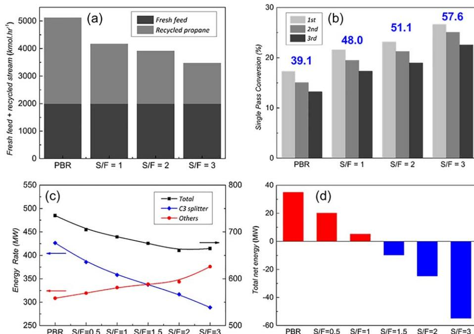
**Figure 9.** (a) Total flow rates entering PBR and PBMR reactor stages at steady state. (b) Single-pass conversions of each reactor stage in simple recycled PDH plant. The numbers in each condition indicate the overall single-pass conversion. (c) Required energy duties of C<sub>3</sub> splitter, other streams, and total streams with respect to S/F ratios. Solid lines are a guide to the eye. (d) Total net energy duty in PBR and PBMRs.
