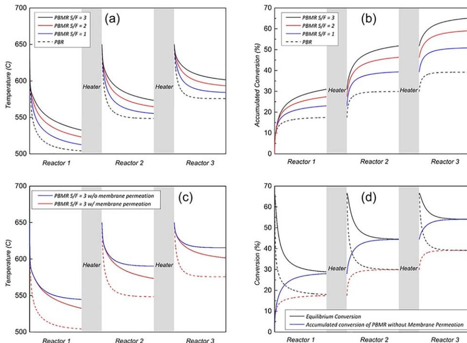
**Figure 6. (a) Temperature profiles and (b) accumulated conversion of three reactor stages (Reactor 1, Reactor 2, Reactor 3) for PBR and PBMR conditions. (c) Temperature profiles of PBMR with and without membrane permeation (S/F = 3). The dashed lines indicate the profiles of PBR. (d) Equilibrium and accumulated conversions along the three reactors using PBMR configuration without membrane permeation (S/F = 3). The dashed lines indicate the equilibrium and accumulated conversions of the PBR.**
