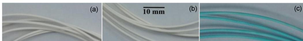
**Figure 1.** Photos of PVDF support membrane (a), PVA coated membrane (b), and PVDF/Cu-BTC membrane (c).
