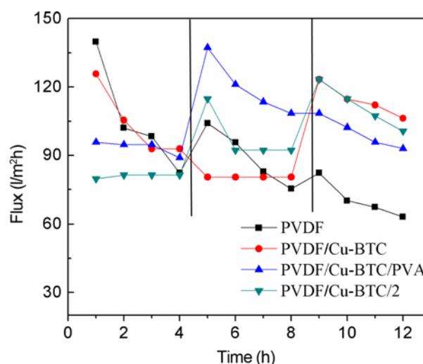
**Figure 7.** Flux changes of the membranes after continuously filtration for 3 days.
