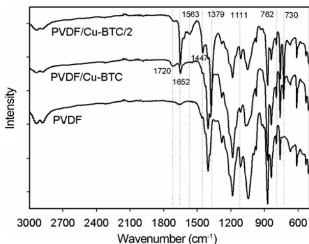
**Figure 3.** FTIR spectra of the membranes.
