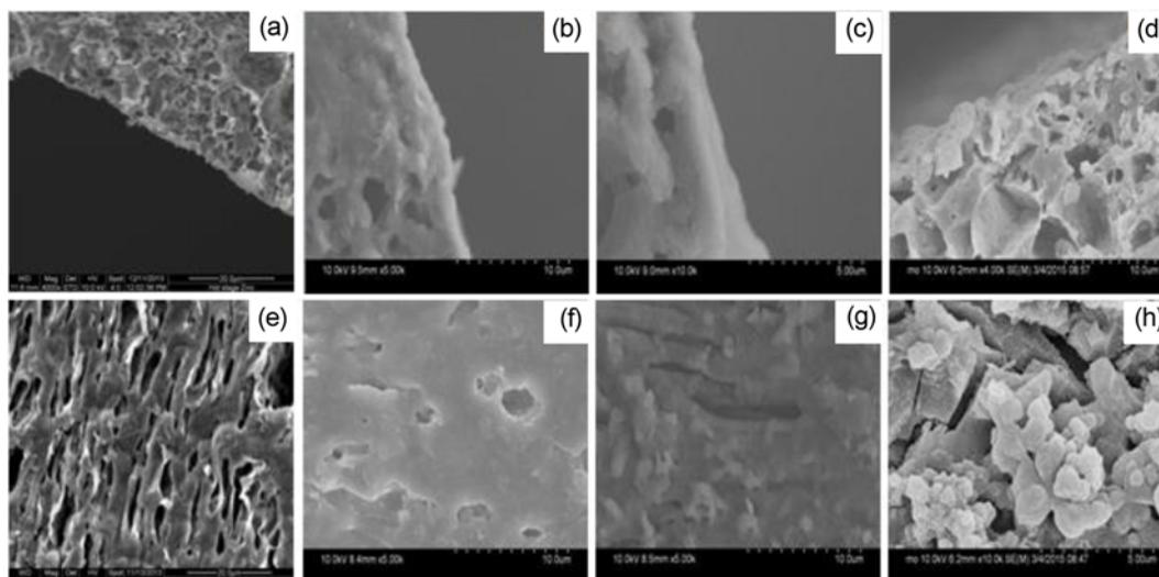
**Figure 2.** SEM images of the membranes. Cross sectional and surface images of PVDF support membrane ((a) & (e)), PVA coated membrane ((b) & (f)), PVDF/Cu-BTC membrane ((c) & (g)), PVDF/Cu-BTC/2 membrane ((d) & (h)).
