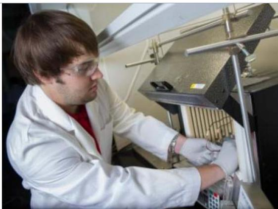
Georgia Tech researcher Andrew Brown places a finished hollow fiber metal-organic framework membrane module into a membrane testing apparatus to measure its gas separation properties.
